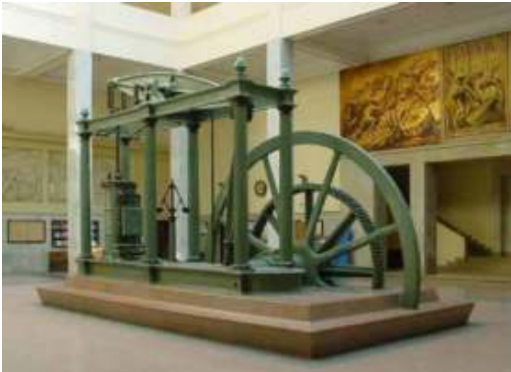
The Heart of the Industrial Revolution: the Watt double-acting steam engine. (Courtesy: Wikipedia, The Free Encyclopedia )
