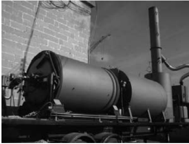
The mobile incinerator procured by the Civil Abattoir to treat fallen animals that fall under category 1 according to the ABP regulation.
